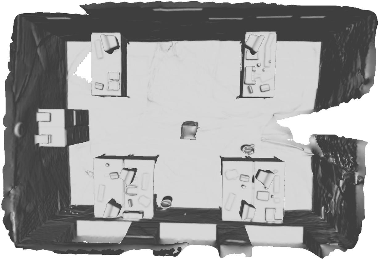
Figure C.3: Reconstruction of the `office_1` sequence from the Augmented ICL-NUIM dataset, as given by our method with the  $L_{\frac{1}{2}}$  loss function
