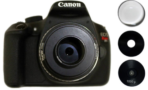
Figure S3. Optical prototype. (Left) Our optical prototype, which consists of a Canon camera and a Thorlabs singlet lens. (Right) Images of the lens and aperture mask for chromatic aberration images, followed by the pinhole mask for all-in-focus images.
