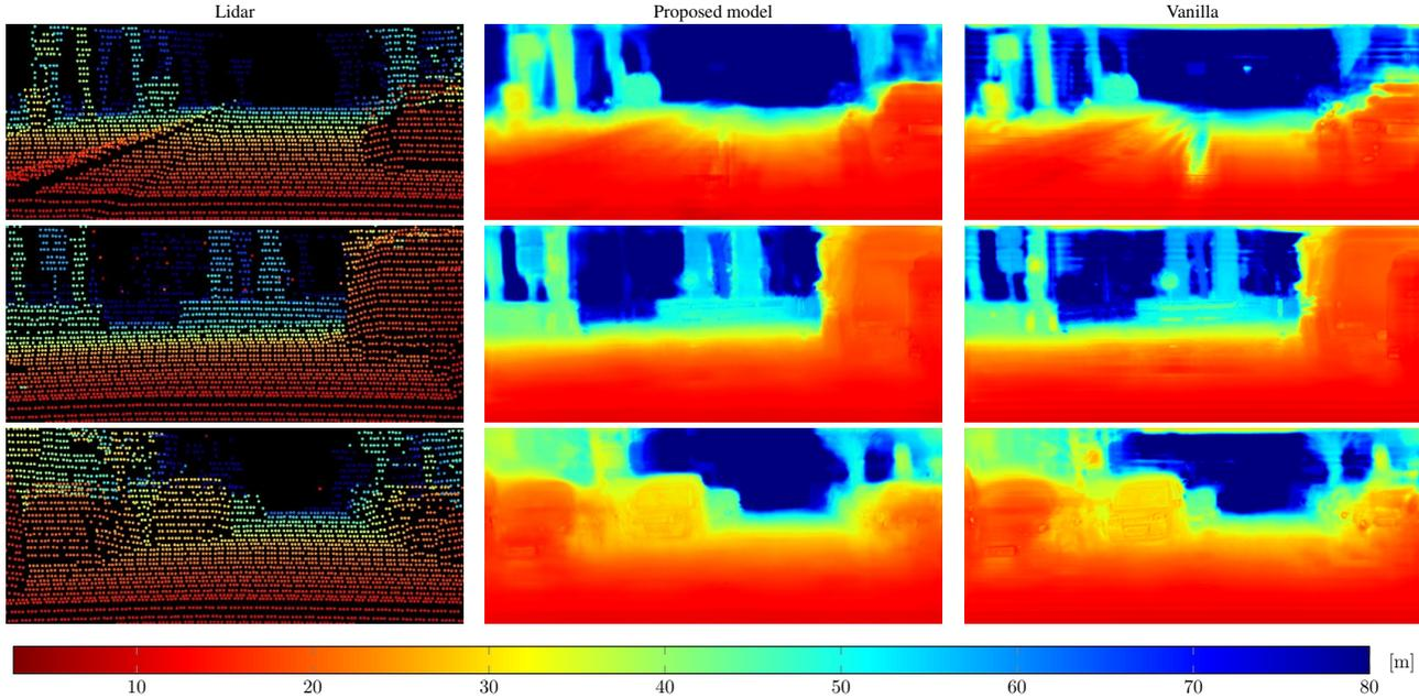
Figure 12: Experimental qualitative results of our proposed model and the vanilla model. Each row show an output for an specific example. The first column illustrates the sparse lidar data of each example
