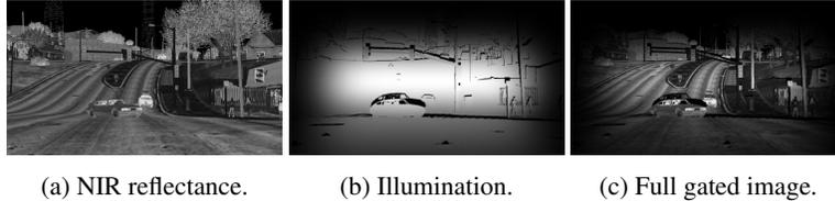
Figure 5: From left to right: heuristically simulated NIR reflectance, laser illumination, combined NIR reflectance and laser illumination.
