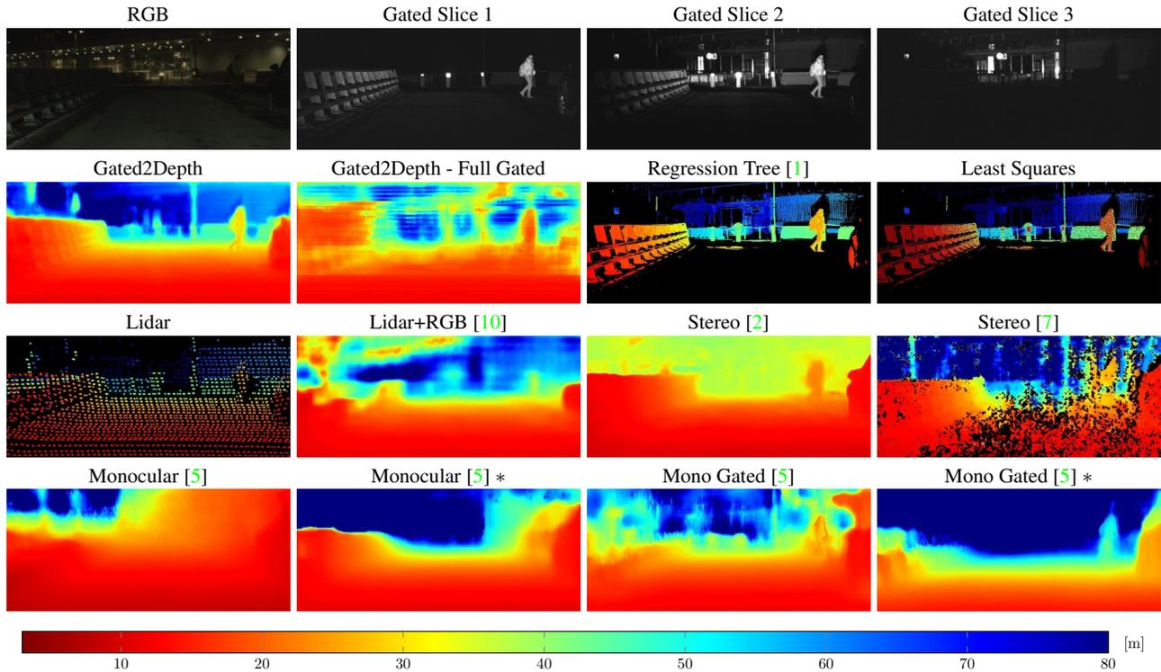
Figure 15: Qualitative results for our method and reference methods over real night time examples. For each example, we include the corresponding RGB and all three gated slices, along with the lidar measurements. Our method generates more accurate and detailed maps over the full depth range in comparison to the other methods.
