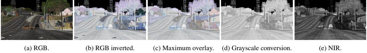
Figure 4: From left to right: original RGB image, inverted RGB image, maximum overlay of original and inverted RGB image, grayscale converted overlay image, final heuristically simulated NIR color model image after gamma correction.
