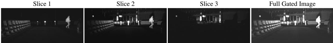
Figure 10: Accumulating three gated slices yields a single unmodulated exposure, full gated image, with continuous illumination.
