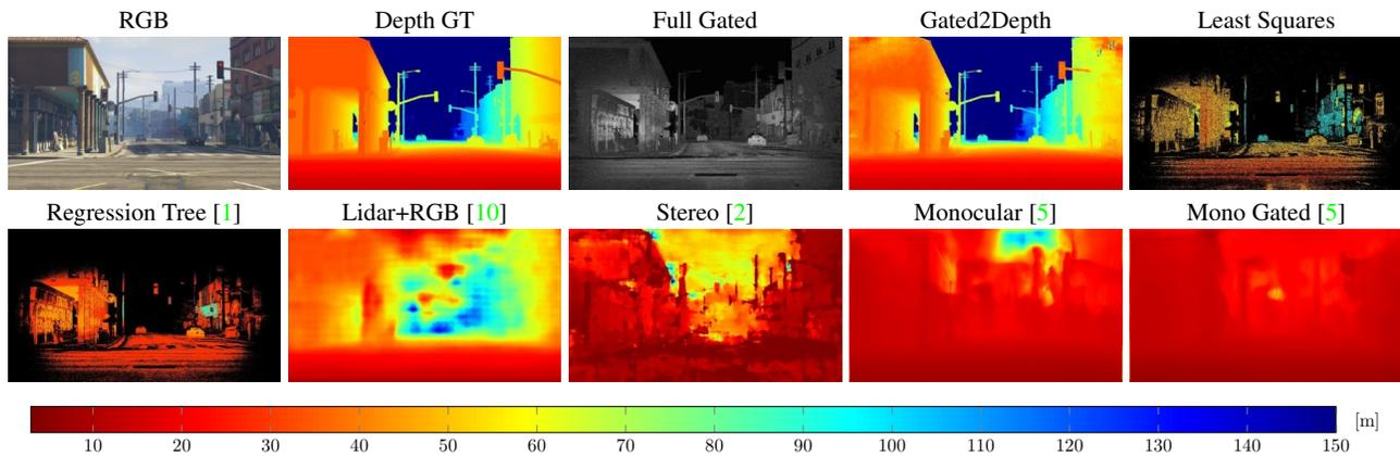
Figure 17: Qualitative results for our method and reference methods over simulated night time examples. For each example, we include the corresponding RGB and full gated image, along with the Depth GT and lidar sampling for training [10]. Our method generates more accurate and detailed maps over the full depth range in comparison to the other methods.
