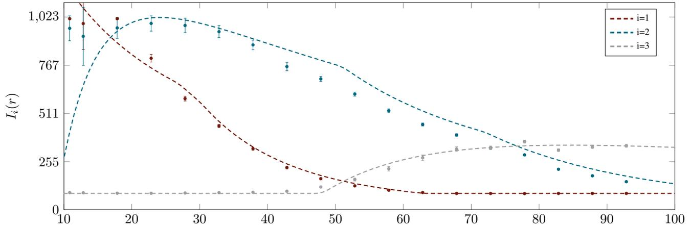
Figure 6: Measurements on a 50 % reflective target of the three range-intensity profiles  $I_i(r)$ ,  $i \in \{1, 2, 3\}$  used in this work, and our modeled range-intensity profiles according to (3) plotted with distance  $r$  [m].
