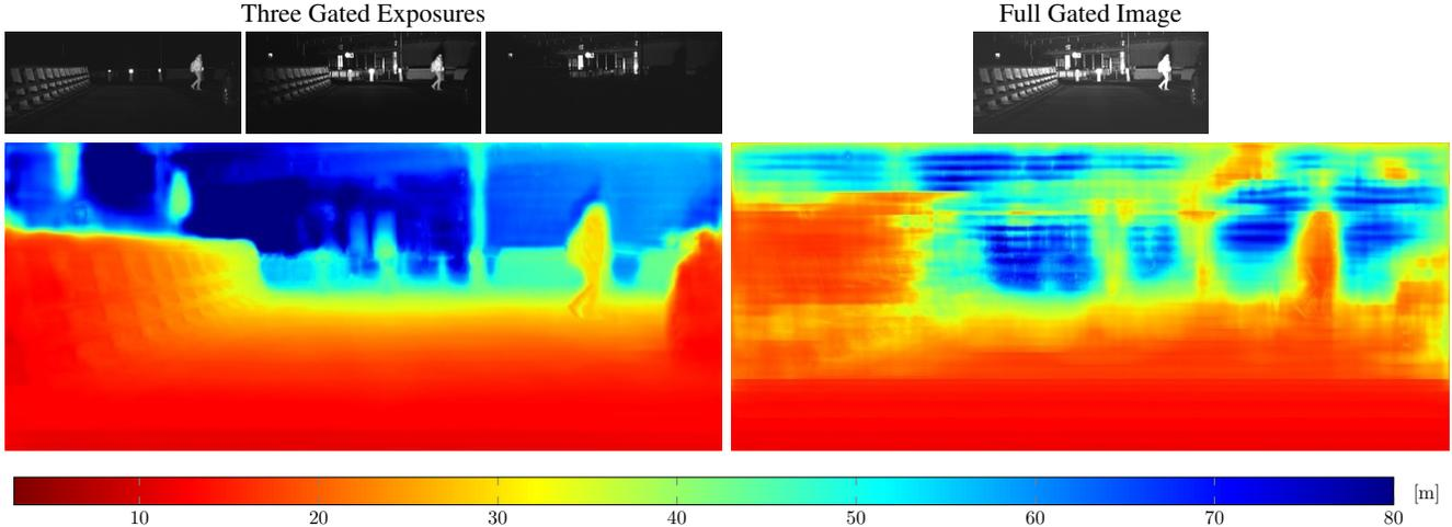
Figure 11: Depth estimation using three gated slices and a full gated image. See Figure 15 for this capture and further comparisons.
