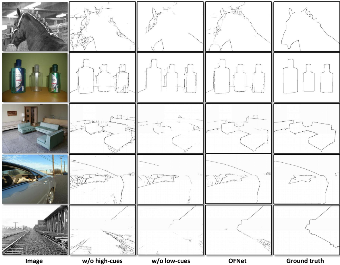
Figure 2: Edge maps of various approaches. Column 1 st : Input image. Column 2 nd – 4 th : OFNet without high-cues, OFNet without low-cues and OFNet. Column 5 th : Ground truth.
