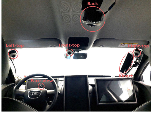
Figure 2: Interior of the simulator depicting the modified dashboard and camera positions.
