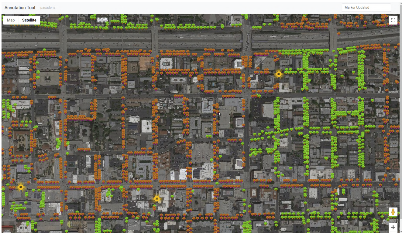
Figure 1: Green tree markers represent trees that are annotated. Brown trees represent annotated labels. Dragging and dropping the tree icon annotates the tree's location by updating it. New trees can be added by clicking the mouse left button in empty areas. Trees can be removed also by the mouse right click.
