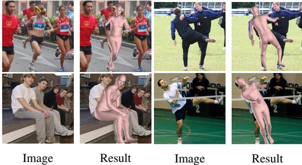
Figure 2: Typical failure cases of our approach. Failures include wrong orientation of the head, confusion because of multiple people in the scene, and mis-alignment between the model and image, particularly for the extremities.
