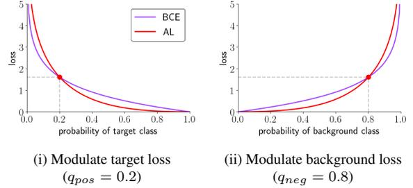
Figure 1. How an anchor probability modulates loss values. When the prediction score of target class is lower than  $q_{pos} = 0.2$ , anchor loss penalizes more than binary cross entropy (i). On the contrary, when the prediction score of background class is higher than  $q_{neg} = 0.8$ , the loss value becomes higher than the binary cross entropy (ii).
