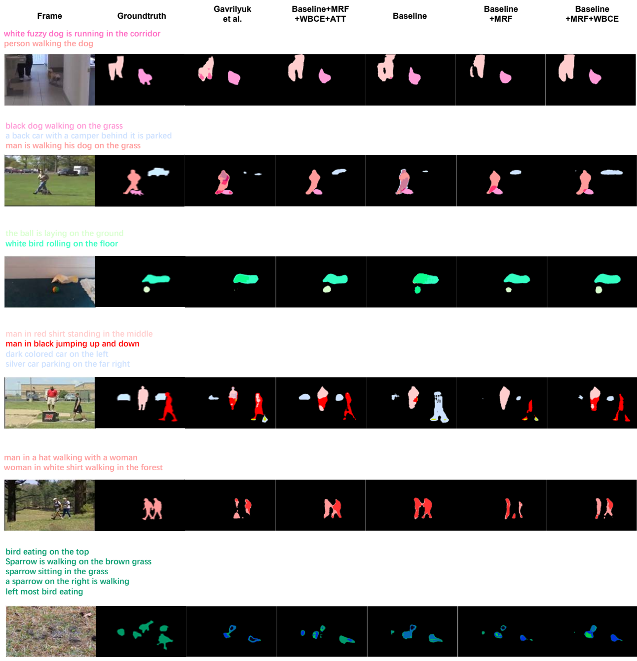
Figure 2. Segmentation results of the frames containing multiple actors and actions. Multi-resolution Fusion, Weighted Binary Cross Entropy with logits, Attention model are abbreviated as “MRF”, “WBCE” and “ATT”, respectively.
