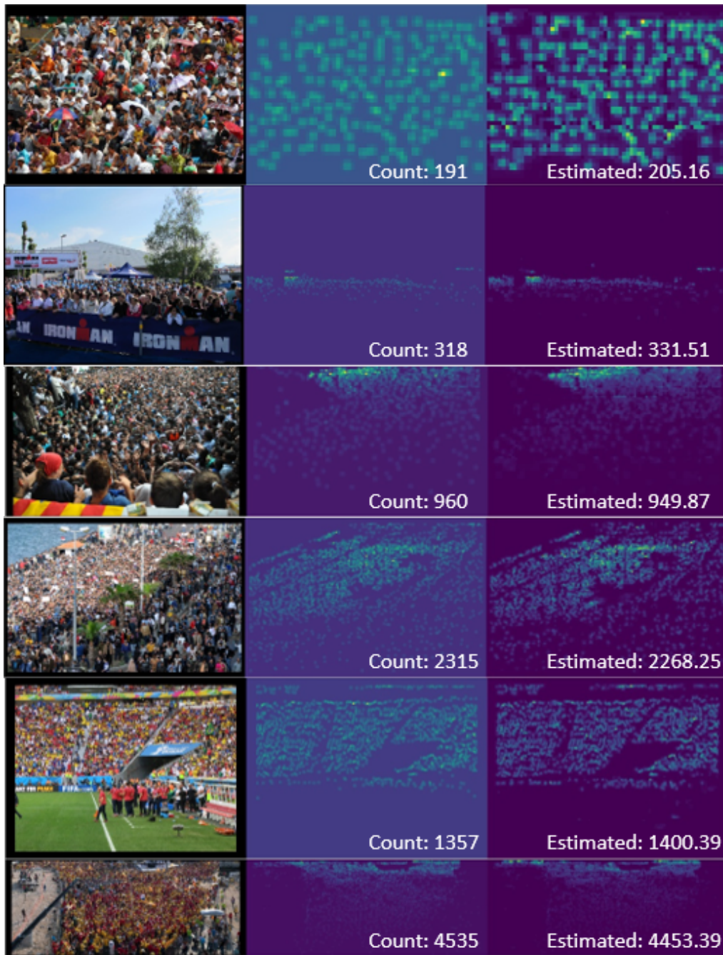
Figure 6. Some samples generated by S-DCNet from the test set of UCF-QNRF dataset. The left column shows the original images, while the middle and right columns display the ground truth and predicted count maps respectively.
