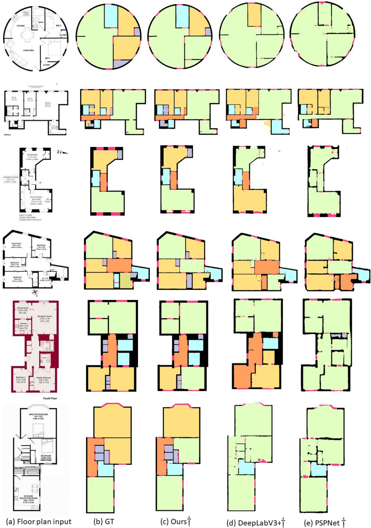
Figure 2. Additional comparison results (2/3) on the R3D dataset by applying (c) our method, (d) DeepLabV3+, and (e) PSPNet to the floor plan inputs shown in (a). GT denotes ground truth. Symbol † indicates the method with our postprocessing.
