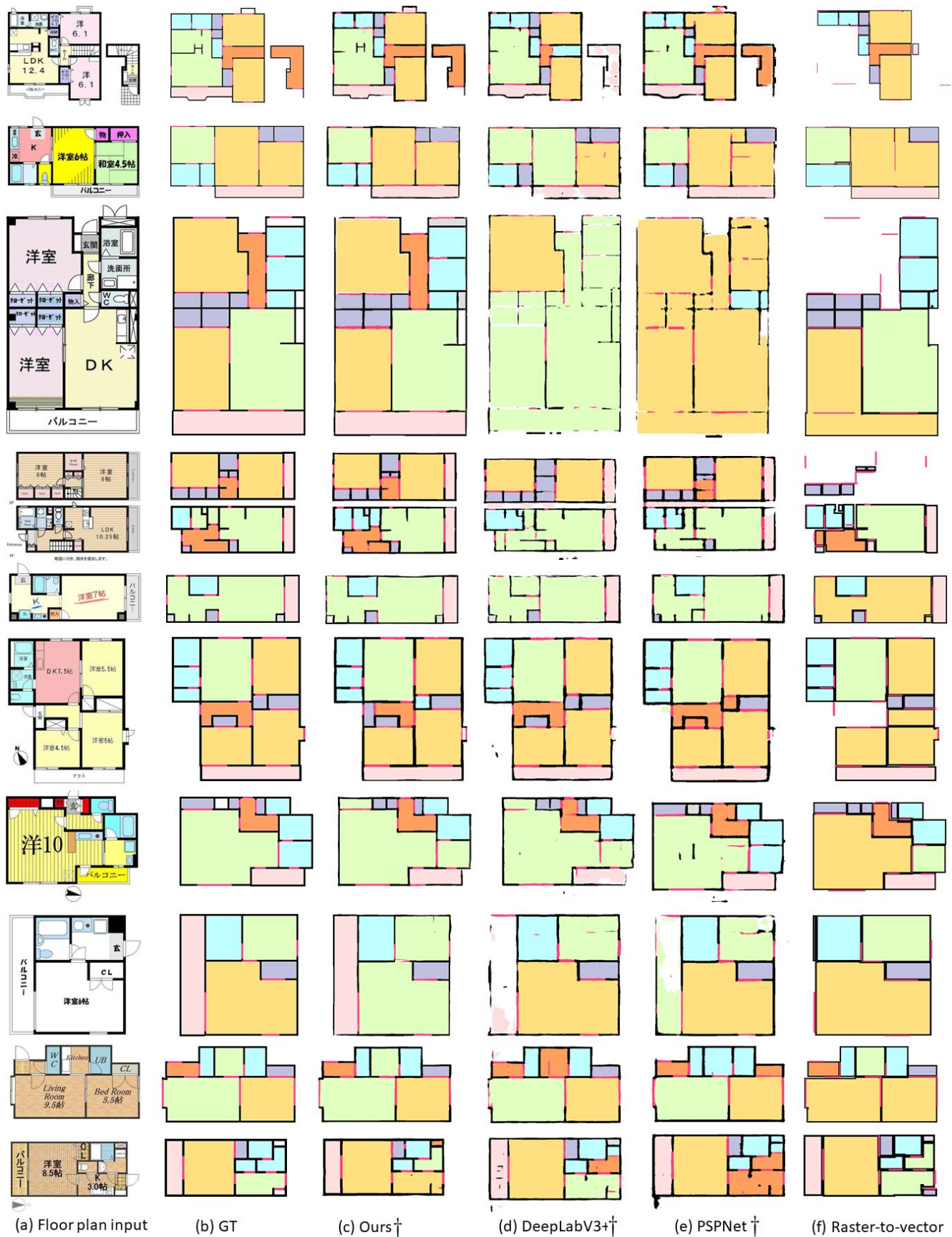
Figure 4. Additional comparison results on the R2V dataset by applying (c) our method, (d) DeepLabV3+, (e) PSPNet, and (f) Raster-to-vector to the floor plan inputs shown in (a). GT denotes ground truth. Symbol † indicates the method with our postprocessing
