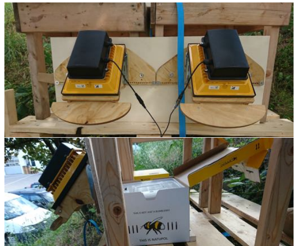
Figure 1. Two monitoring systems are attached to individual bumblebee hives. Bumblebees are filmed at the hive entrance.
