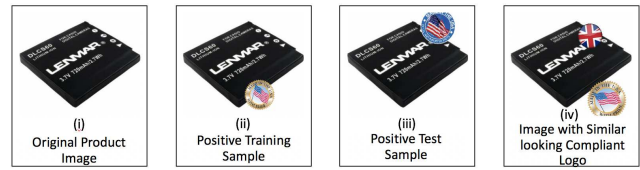
Figure 8. Step d: Used training logo (top-left from figure 7) and applied random scaling, rotation and translation to generate a positive training sample as image (ii). Similarly, testing logo (top-right from figure 7) used to generate a test sample as image (iii). Image (iv) - Use similar-looking compliant logos collected in step b for superimposition.
