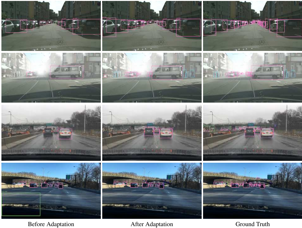
Figure 5. Examples of the detection results from our three adaptation tasks. The first two rows are the tasks KITTI → Cityscapes and Cityscapes → Foggy Cityscapes respectively, while the last two rows are the task Cityscapes → BDD100k. We show the detection results on the target domain before and after applying our adaptation method as well as the ground truth labels.
