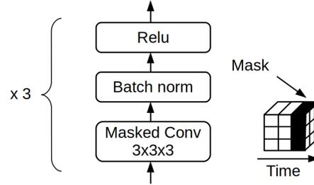
Figure 2. Details of the main autoregressive architecture. It is composed of 3 layers of temporally masked 3D convolutions separated by batchnorm and relu.
