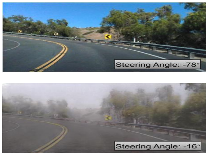
Figure 1: Steering Angle(radians) deviation seen in the same scene due to Fog, for the AutoPilot model[8]. Lower image was generated by our method given the left image
