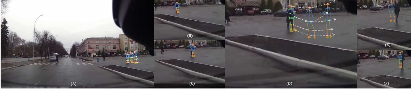
Figure 8: Qualitative pose prediction results. (A) the t_p = 15 length input sequence of poses. (B) and (C) the cropped frames with the pedestrian and the corresponding filled in pose at the start and end of the input sequence. (D) the prediction pedestrian locomotion for the next t_f = 15 frames. (E), (F) the predicted poses at the start, intermediate, and end of the output sequence, respectively. Video visualizations are available at: https://karttikeya.github.io/publication/plf
