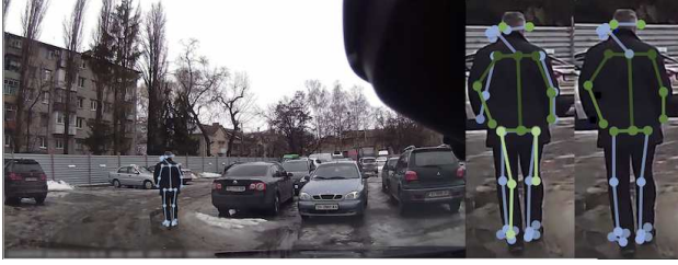
Figure 6: Qualitative results showing the results of pose completion (Section 3.2). From left to right: denoised pose, cropped version of the same pedestrian with the original OpenPose output (green), denoised pose (blue).
