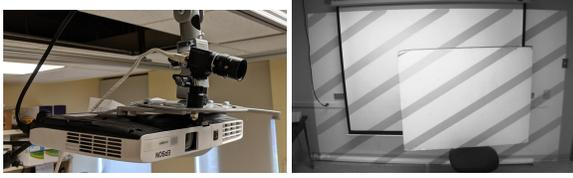
(a) Vertically aligned projector and camera (b) Substantially overlapping fields-of-view
