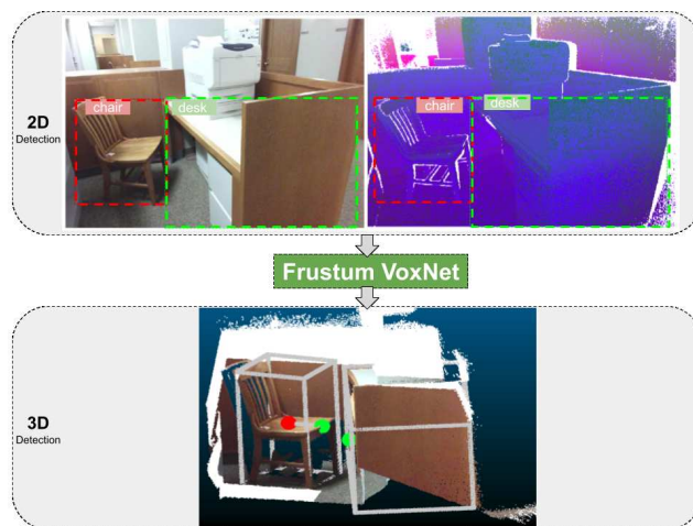
Figure 1. Overview of the whole system. Upper left: RGB image and detected 2D bounding boxes. Upper right: DHS (Depth Height and Signed angle) image, and detected 2D bounding boxes. A DHS image is a pseudo-RGB image generated by a depth image (see text). Bottom: The final 3D detected objects from the associated 3D range image. The 3D detection not only provides an amodal bounding box but also an orientation. The red point is the center of the bounding box and the green one is the front center. The detected 2D bounding boxes from either an RGB or DHS image, generate 3D frustums (which are prisms having as apex the sensor location and extend through the 2D bounding boxes to the 3D space). They are then fed to our Frustum VoxNet network, which produces the 3D detections.
