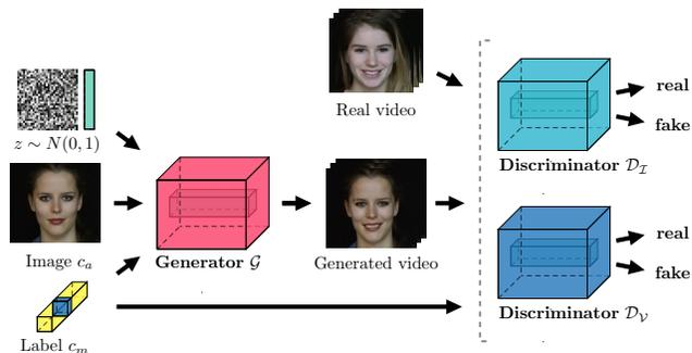
Figure 1: The proposed ImaGINator architecture incorporates Generator  $G$ , image Discriminator  $D_I$ , as well as video Discriminator  $D_V$ .  $G$  accepts  $c_a$ ,  $c_m$  and noise as input, and seeks to generate realistic video sequences. While  $D_I$  discriminates whether the generated images contain an authentic appearance,  $D_V$  additionally determines whether the generated videos contain an authentic motion.
