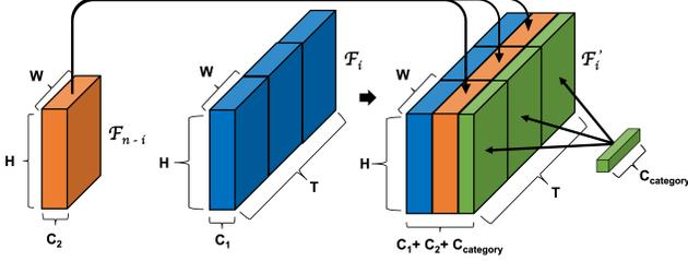
Figure 3: **Spatio-temporal fusion.** Blue and orange cuboids represent the intermediate feature maps in the Decoder and Encoder respectively. Our proposed fusion scheme enforces the Decoder reutilizing spatial information through skip connections. Based on such operations, temporal consistency can be modeled in multi-levels.
