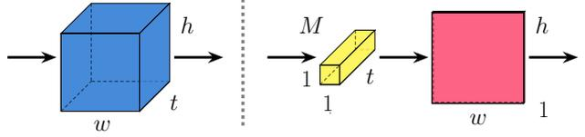
Figure 4: **Transposed 3D convolution** (on the left) vs. **proposed Transposed (1+2)D convolution** (on the right). The transposed 3D convolutional filter of size  $t \times w \times h$  has been decomposed into  $M$  transposed 1D temporal convolution filters  $t \times 1 \times 1$  and a transposed 2D spatial convolution  $1 \times w \times h$ . The operation  $M$  denotes the number of 1D filters,  $t$  indicates the temporal size, and  $w$  and  $h$  indicate the spatial size.
