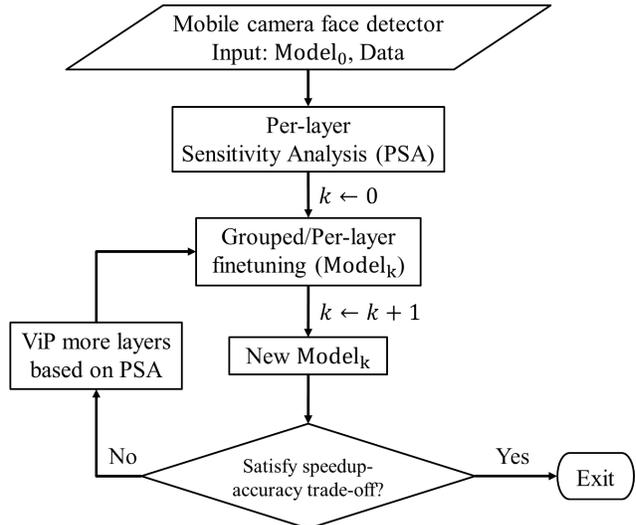
Figure 1. An example of applying ViP to the mobile phone camera face detector. ViP progressively generates new models with higher speedup until we obtain the model that best satisfies the requirement on speedup-accuracy trade-off.
