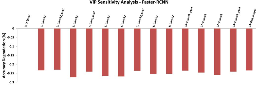
Figure 4. ViP sensitivity analysis of faster-rcnn with VGG16 backbone under PASCAL VOC 2007 dataset. For each of the conv layers, we insert ViP immediately after it, and evaluate the accuracy without finetuning. The sensitivity is measured as the accuracy degradation.
