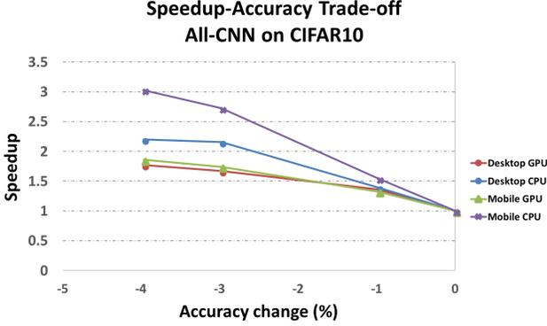
Figure 2. Speedup-Accuracy trade-off obtained by applying ViP on All-CNN model with CIFAR-10 dataset.
