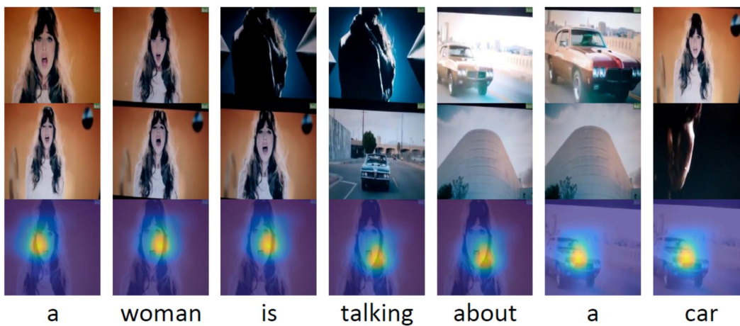
Figure 3. Failure case: the system fails to recognize the sound. The 14 frames in the first two rows show the temporal sequence of the video. The 3rd row shows the frames selected by our TS model for each word in the generated caption, overlaid with its corresponding spatial attention map.
