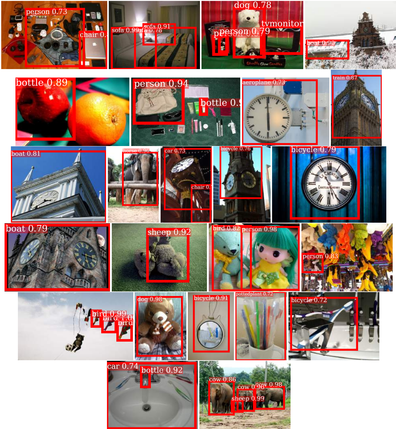
Figure 1: MISDETECTIONS FROM FASTER R-CNN These results are from the Faster R-CNN network used in our paper. The network was trained on the PASCAL VOC 2007-2012 training and validation set while the above images belong to MSCOCO dataset. Ideally, the network was supposed to reject all the above detections as background.
