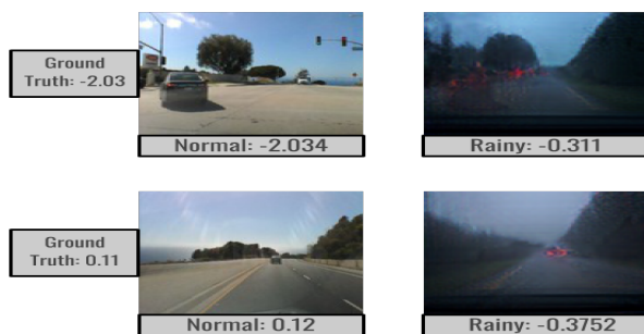
Figure 8: Rainy counterparts of the original images (right) generated using our model trained on Sully Chen with a single rainy video taken from YouTube. The ground truth and predicted steering angles (in radians) in both cases are given alongside.
