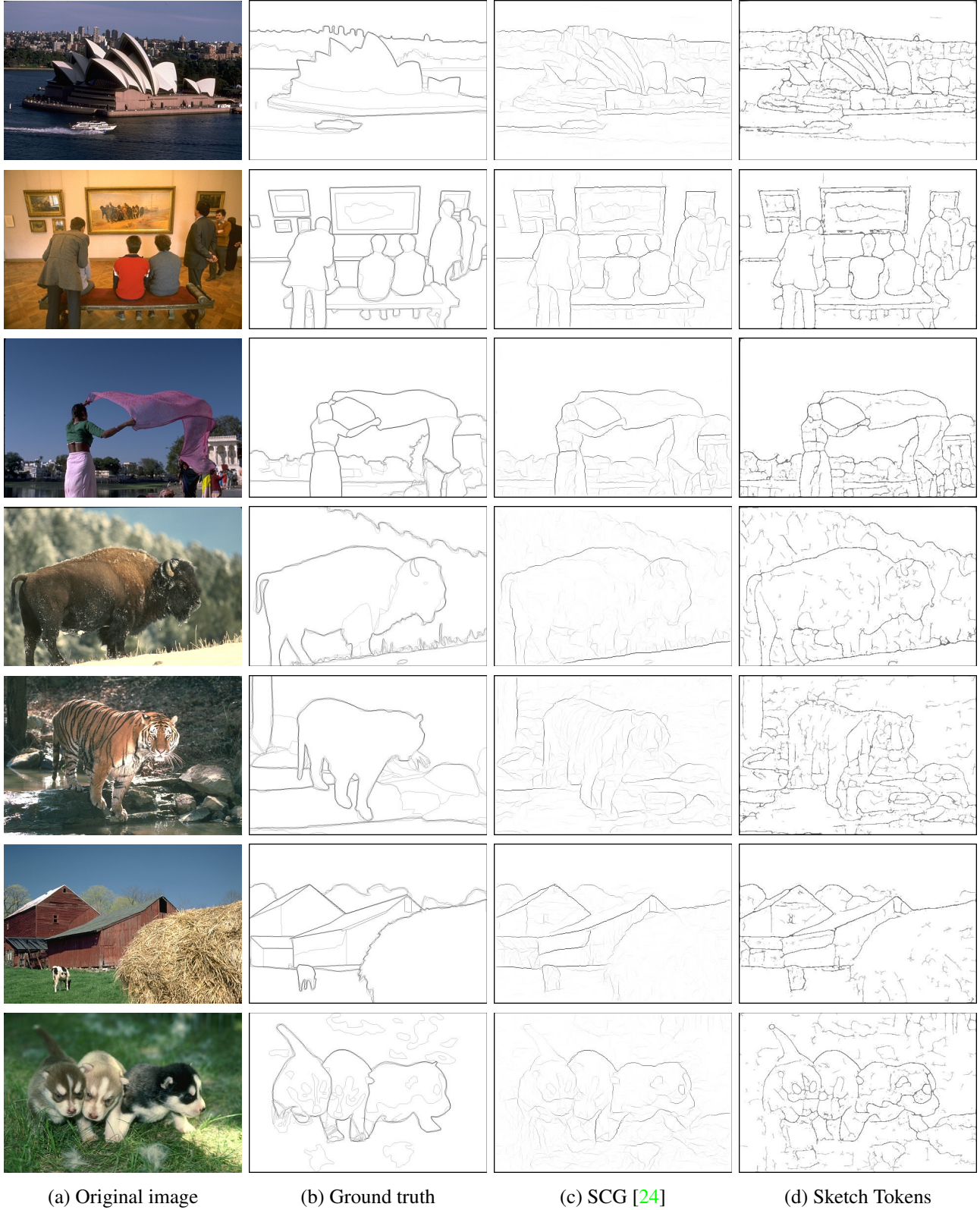
Figure 10. Examples of contour detection on the BSDS500 [1]. For Sketch Tokens we define edge strength according to Equation 2 and apply smoothing and standard non-maximal suppression to obtain peak edge responses [3]. Note how our method captures finer details such as the structure of Sydney Opera House on the 1st row and human legs on the 2nd row.
