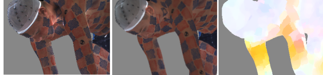
Figure 7: Sliding analysis using optical flow. We compute the optical flow between real images (first column) and synthetic ones (second column). Vertices mapped to pixels with high flow magnitude are deemed misaligned.
