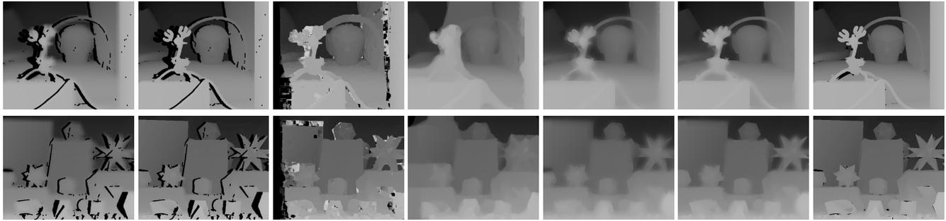
Figure 4. Experimental results on the two stereo pairs from the Middlebury dataset. From left to right: Input depth maps having (a) Reduced and (b) Original resolution. Depth maps resulted from (c) ENCC [28], (d) LDOF [7], (e) M-D using (a) as input, and (f) M-D using (b) as input. (g) Ground truth. For the best visual evaluation, it is recommended to enlarge the figure in the electronic version of this article.
