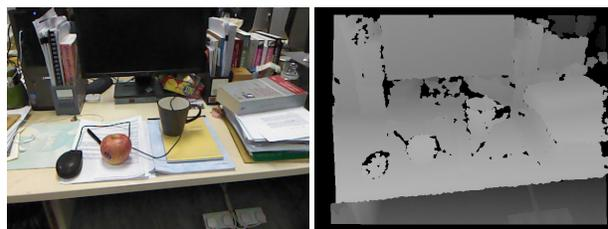
Figure 1. A RGB-D frame from a Kinect consists of a color image and a depth map of the scene. Light intensities in the depth map correspond to surfaces that are close to the camera, while dark intensities correspond to surfaces that are far away from the camera.
