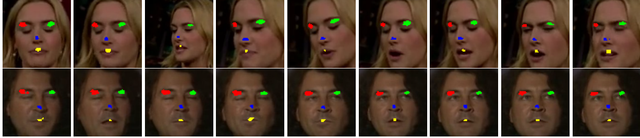
Figure 1. Unsupervised GMM implicitly performs robust face part tracking. On the left frame of the track in the top row , we manually selected 4 points on eyelids, nose and mouth. These points correspond to 4 SIFT patches, which are assigned to particular Gaussians from the GMM (colour-coded with red, green, blue, and yellow). We visualise the pixels assigned to these Gaussians on 9 frames of the track. As can be seen, the same face parts get consistently assigned to the same Gaussians, which indicates the robustness of the representation with respect to the face position variation. In the bottom row , we visualise the face pixels assigned to exactly the same Gaussians as in the top row, but for a different person. Again, they correspond to the same face parts, which means that the assignment is consistent across different identities. The comparison of Fisher vectors thus can be seen as the implicit and robust comparison of face parts.
