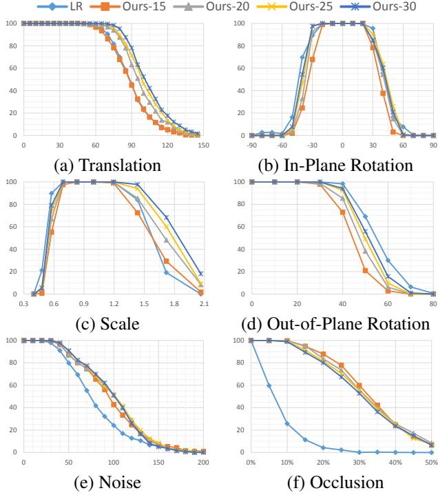
Figure 2. These plots show the tracking robustness of our algorithm with varying  $n_r$  (15, 20, 25, 30) and compare it with Linear Regression (LR) [13] under different (a-d) transformations, (e) levels of Gaussian noise and (f) percentage of occluded region.
