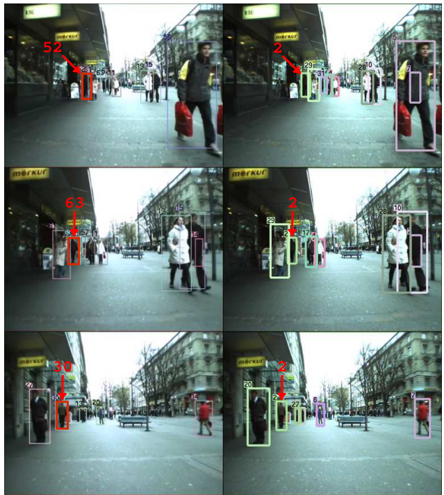
Figure 3. Columns 1 and 2 compare the tracking results of LRM-CNF [5] (left) and our approach (right) respectively on the ETH BAHNHOF sequence (frames 104 - first row, 130 -second row, 187- third row). Note the detection windows pointed by red arrows. We can see that our approach maintains ID labels more reliably.
