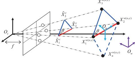
Figure 1. A diagram illustrating the PnP problem.
