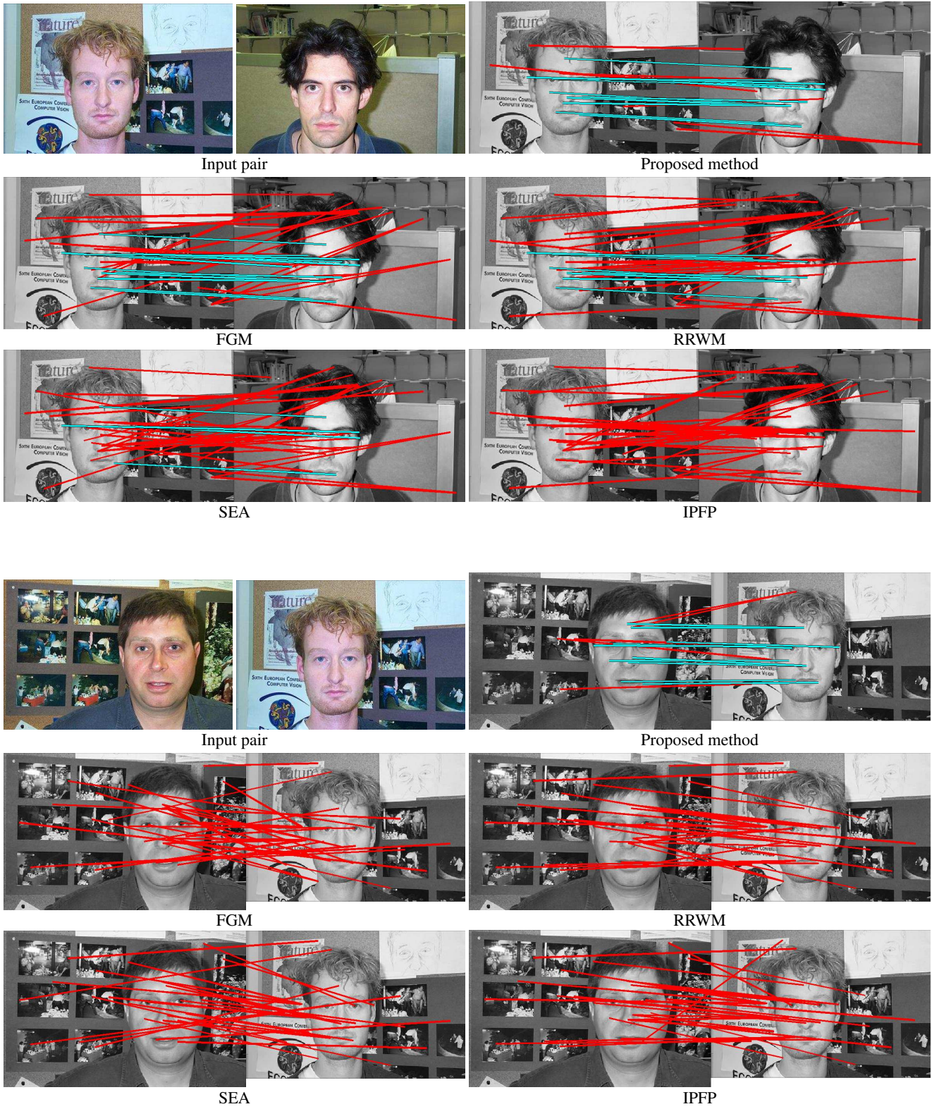
Figure 2. Example results of the real image matching using local features. True positive matches are represented by cyan lines, and false positive matches are represented by red lines.
