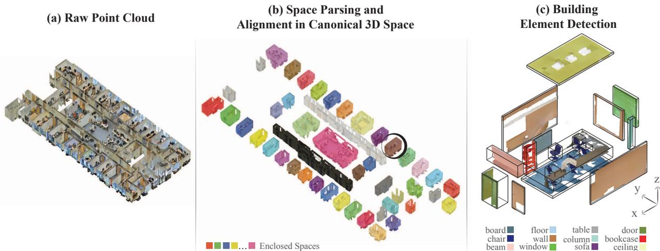
**Figure 1: Semantic parsing of a large-scale point cloud.** **Left:** the raw point cloud. **Middle:** the results of parsing the point cloud into disjoint spaces (*i.e.* the floor plan). **Right:** the results of parsing a detected room (marked with the black circle) into semantic elements.
