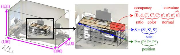
Figure 4. **Detection box in the unit cube reference coordinate system and features for a sample object (table).** Our features are the detection anchor point, size and features of each sub-box. Features of non-occupied voxels are 0 (see Table 1 for all features).
