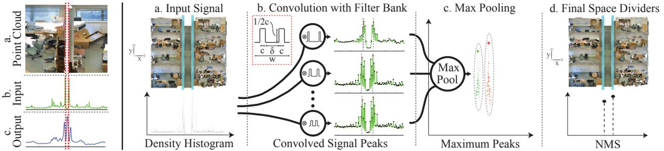
Figure 2. **Left:** Convolution of the devised filter with the histogram signal. The Histogram signal along axis  $x$  is the histogram of  $x$  coordinates of all points. **Right:** Space divider detection algorithm. We start with the density histogram signal (a), convolve it with the filter bank (b), and perform max-pooling (c) to identify the space dividers (d).
