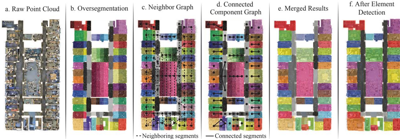
Figure 3. **Merging the over-segments:** We start with a set of over-segments (b) generated from the point cloud (a) and create their neighbor graph (c). Then, we merge nodes (d-e) as explained in Sec. 3.1.2. We update (f) the results given the output of element detection (Sec. 4.2).
