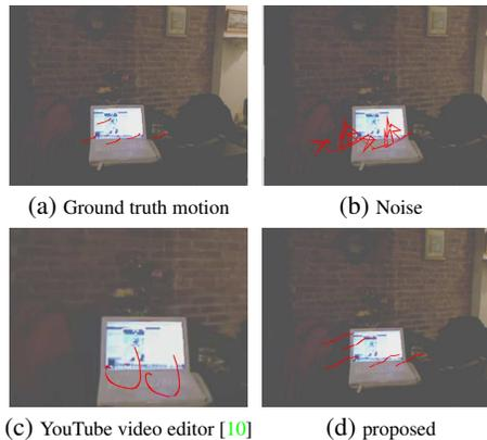
Figure 8: Video stabilization. We used the “NYUv2-living room part 1-living room 0009” dataset. Features are tracked between frames 265 and 285. The feature trajectories are overlaid as red polylines on frame 285.
