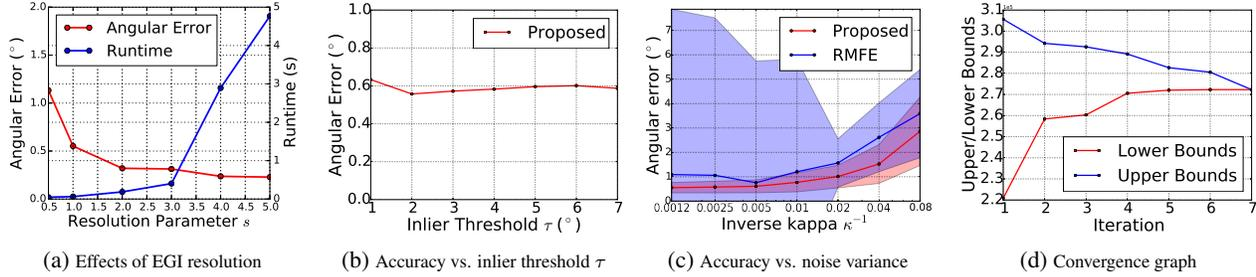
Figure 5: Simulation results for observing the behaviors of the proposed method.
