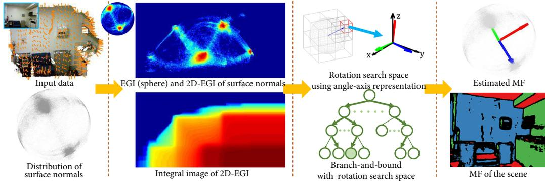
Figure 1: Overview of the proposed MF estimation approach. *First column*: Input data and distribution of surface normals of a scene from NYUv2 dataset [24]. *Second column*: Its surface normal histogram, *i.e.*, EGI, the 2D-EGI and its integral image to efficiently calculate bounds. *Third column*: Illustration of the efficient bound based BnB framework using rotation search space. *Last column*: The estimated globally optimal MF.
