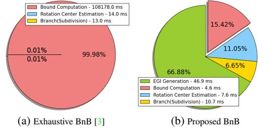
Figure 6: Time profiles of the exhaustive BnB [3] and the proposed BnB approach.
