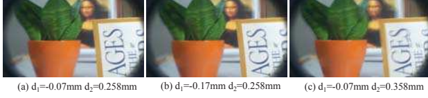
Figure 8. The refocusing images under different d_1, d_2 . (a)(b) have 0.1 difference in d_1 , (a)(c) have 0.1 difference in d_2 .
