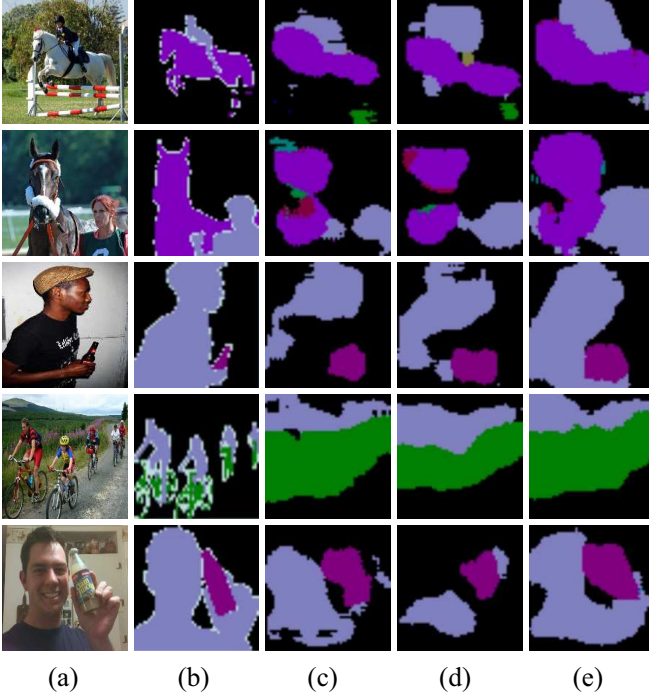
Figure 6. Visualized semantic labeling results. (a) The input images; (b) The groundtruth labeling results; (c) Our proposed method (weakly-supervised); (d) Deeplab(weakly-supervised) [20]; (e)MIL-ILP(weakly-supervised) [22]
