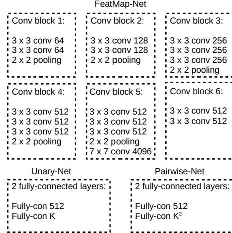
Figure 6. The detailed configuration of the networks: FeatMap-Net, Unary-Net and Pairwise-Net.  $K$  is the number of classes. For FeatMap-Net, the top 5 convolution blocks share the same configuration as the convolution blocks in the VGG-16 network. The stride of the last max pooling layer is 1, and for the other max pooling layers we use the same stride setting as VGG-16.
