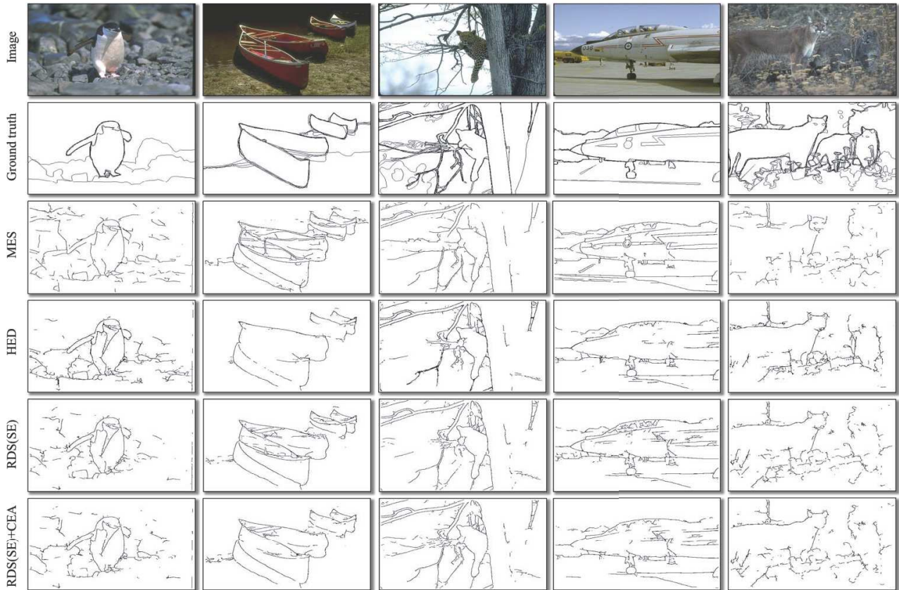
Figure 9: Illustration of five edge detection examples. The first and second rows list the original image and its ground truth. The third and fourth rows display the results from MES [34] (Threshold=.407) and HED [39] (Threshold=.320). The proposed RDS(SE) (Threshold=.390) and RDS(SE)+CEA (Threshold=.347) methods are shown in the fifth and sixth rows. Compared with HED [39], RDS can reduce the false positives, such as the stones in the first image. Meanwhile, our method can obtain more true positives, for example our closed boundaries of the boats in the second image.
