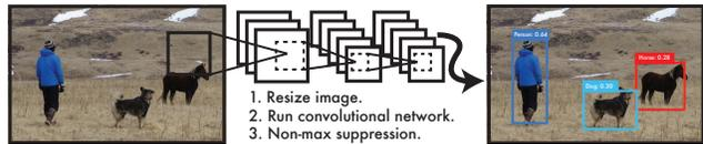
**Figure 1: The YOLO Detection System.** Processing images with YOLO is simple and straightforward. Our system (1) resizes the input image to  $448 \times 448$ , (2) runs a single convolutional network on the image, and (3) thresholds the resulting detections by the model’s confidence.
