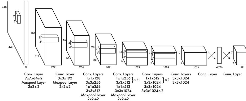
**Figure 3: The Architecture.** Our detection network has 24 convolutional layers followed by 2 fully connected layers. Alternating  $1 \times 1$  convolutional layers reduce the features space from preceding layers. We pretrain the convolutional layers on the ImageNet classification task at half the resolution ( $224 \times 224$  input image) and then double the resolution for detection.
