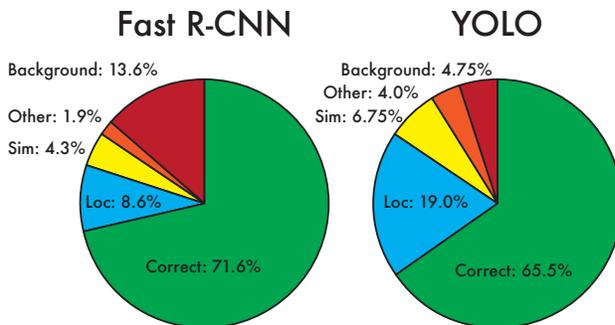
**Figure 4: Error Analysis: Fast R-CNN vs. YOLO** These charts show the percentage of localization and background errors in the top N detections for various categories ( $N = \#$  objects in that category).
