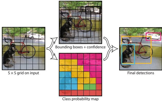
**Figure 2: The Model.** Our system models detection as a regression problem. It divides the image into an  $S \times S$  grid and for each grid cell predicts  $B$  bounding boxes, confidence for those boxes, and  $C$  class probabilities. These predictions are encoded as an  $S \times S \times (B * 5 + C)$  tensor.
