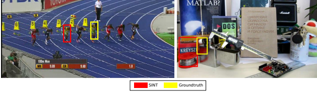
Figure 5: Failure cases of SINT: similar confusing object (left) and large occlusion (right). Examples are from OTB sequences ‘Bolt’ and ‘Lemming’ respectively. In the left example, the tracker fires on another Jamaican runner in the same uniform as the target. In the right example, the target is heavily occluded by the lighter.
