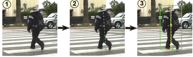
Figure 2: Illustration of bounding box generation for human baseline. The annotator only needs to draw a line from the top of the head to the central point between both feet, a tight bounding box is then automatically generated.
