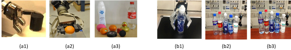
Figure 5. The used robot hands and the grasping objects in SD , SPR and BDH . (a1) The 3-finger Schunk Dextrous Hand (SDH); (a2) The 2-finger Schunk Parallel Hand (SPH); (a3) Objects in SD and SPR : Rubber ball, Balsam bottle, Rubber duck, Empty bottle, Full bottle, Bad orange, Fresh orange, Juggling ball, Tape, and Wood block. (b1) The BH8-280 Hand; (b2) Bottles without water; (b3) Bottles with water.
