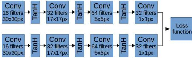
Figure 2. CNN architecture.
