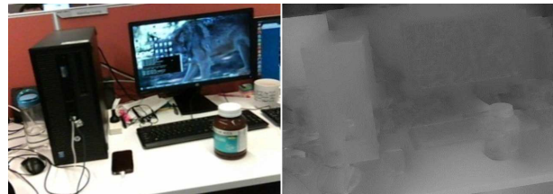
Figure 1. The proposed method builds a complete dense depth map for a monocular camera. Our method combines the robustness and accuracy of dense mapping with efficient sparse patch tracking techniques. Left: image from video. Right: dense depth result.
