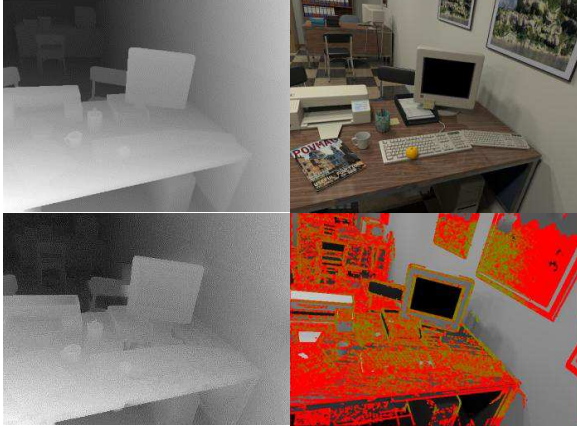
Figure 5. The first row is ground truth(left) and original image(right); the second row is the result of CD-SLAM(left) and LSD-SLAM(right). LSD-SLAM only has depth on yellow and red regions.
