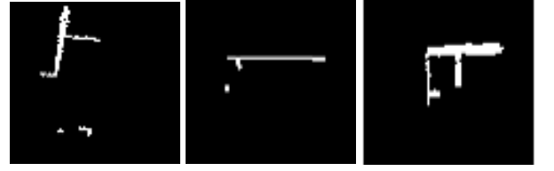
Figure 6. An illustration of point cloud projection. (a) Projection on the XY plane. (b) Projection on the YZ plane. (c) Projection on the XZ plane.
