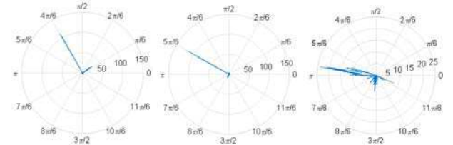
(b) Three direction angle histograms of the rotated point cloud. Figure 4. An illustration of the direction angle histograms. (Figure best seen in color.)
