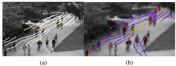
Figure 5: Anomaly Detection. We also evaluate other datasets like UCSD. Trajectories of 63 real pedestrians are extracted from a video. One person in the middle walks against the flow of crowd. Our method can capture the anomaly of this pedestrian’s behavior or movement by comparing the behavior features with those of other pedestrians.
