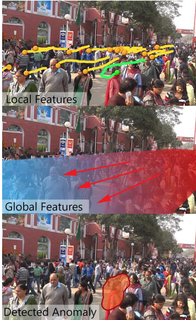
Figure 2: The Anomaly Detection In this example, we see that one pedestrian (marked with green) suddenly makes a U-turn (local feature) in a crowd where everyone is walking in a specific direction/field (global feature). Our system detects this as an anomaly (Refer to Section 3.8).
