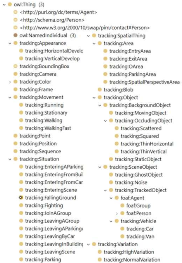
Figure 3. Classes of the Tracking Ontology
