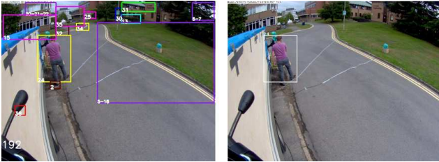
Figure 6. Left image: output of the tracking algorithm with a lot of blobs produced by the camera moving; right image: output of the semantic annotation component applying filtering rules
