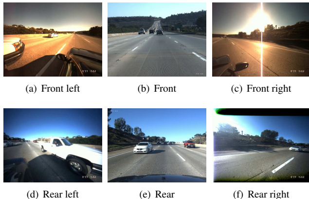
Figure 3. Sample images captured from the synchronized multi-perspective setup. Note the challenges of e.g. glare, shadows, and distortion.
