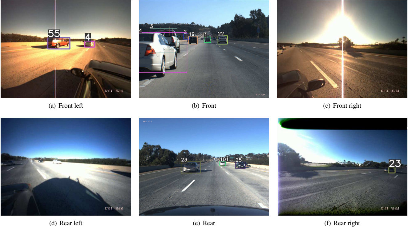
Figure 7. The six perspectives of Seq2 at frame 506. The multi-perspective tracked vehicles are shown by their latest detection in colored bounding boxes with corresponding identification number. Note some vehicles can be seen in multiple perspectives due to overlap, thus assigned the same identification number.
