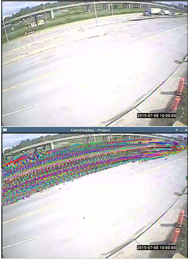
Figure 9. Top: Views of site 032 with, in order from bottom to top, two eastbound lanes, two westbound lanes, one westbound highway entry lane and two westbound highway lanes. Bottom: Westbound highway and entry lanes trajectories.
