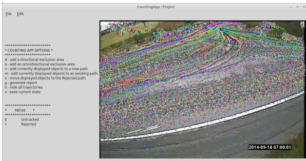
Figure 1. The CountingApp start-up screen showing all trajectories on a video frame background
