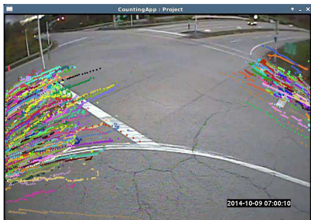
Figure 7. Trajectory fragmentation because of stop-and-go motion of vehicles at the approach of a stop sign (site 028)
