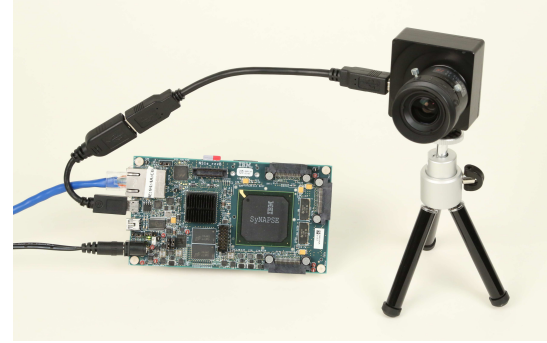
Figure 1: Picture of the setup. The DVS128 camera is connected to the NS1e board using a USB cable. The board exhibits a power cord and an Ethernet cable.
